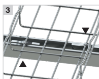
Add an additional FS41 on the opposite side of the channel support for secure installation.
