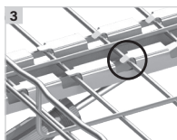
From the underside, depress several tabs using a screwdriver or pliers to secure tray
